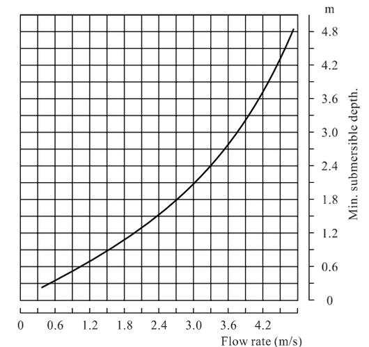
$$\text{Flow rate (m/s)} = \frac{\text{Flow(m}^3\text{/h)}}{\text{Section surface of the pipe(m}^2\text{)}}$$
